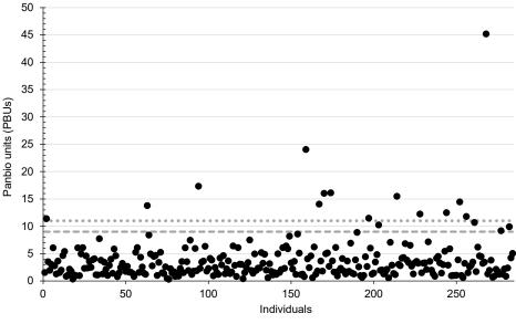
Note: The negative cutoff value (9 PBUs) and the positive cutoff value (11 PBUs) are indicated with dashed and dotted lines (respectively). The intervening values are considered equivocal.
